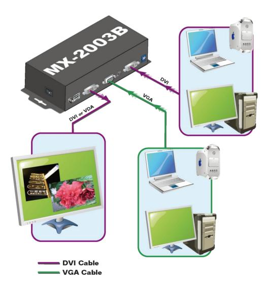
**Figure 1: Configuration Diagram**
